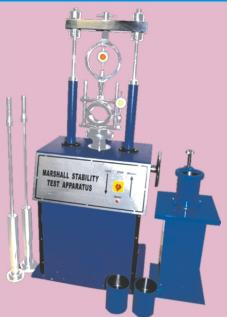
A handle is provided for manual operation during calibration etc. The load frame is fitted with ON OFF, Reversing switch and power indicator lamp in front. Suitable to work on 230V, 50 Hz, AC single phase.
